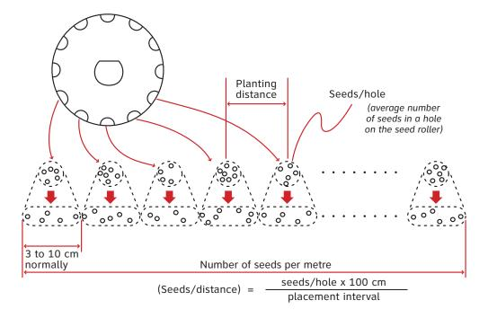
**Caution:** the planting distance depends on the combination of sprocket teeth (11 adjustment positions) and the number of holes on the metering roll. The drive wheel may slip depending on soil quality and placement speed. Therefore, the number of seeds is a guideline only.
