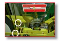
**3** Place the row marker, screw the fixing paws, and then screw the side bolts.
