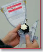
• To remove the pin, turn it as shown in photo below and pull, to release the pin and the roller.
