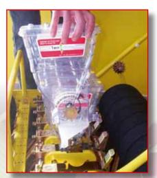
3 Unscrew the white knob and open the retractable portion of the hopper
