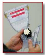
4 To remove the pin, turn it as shown in photo below and pull, to release the pin and the roller.
