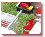
6 Choose the end fitting the most adapted to your needs and install it at the bottom of the fertilizer hopper in the slide rail.
