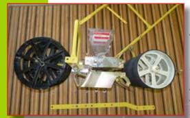
Unscrew and take off each bolt, nut, washer, so that you can release the frame side bar.
