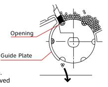
→ SEEDING DISTANCES: The distances between the seeding can be adjusted by adjusting the pinions and the number of holes in the roller, see the seed distance table.
